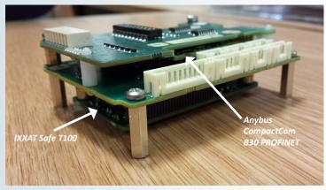
What safety looks like. The IXXAT Safe T100 implements the PROFIsafe layer and the safe control of three dual-channel inputs, as well as one dual-channel output. The Anybus CompactCom handles the unsafe communication and routes the safety communication to the IXXAT T100 via the black channel.
